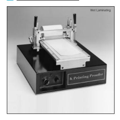
Both wet and dry laminated samples can be produced on the machine using the gravure head with K-Lam laminating accessories. Thes accessories include a rubber covered bed and wired K-Lam bars which are fitted in place of the doctor blade assembly to control adhesive coating weight.
